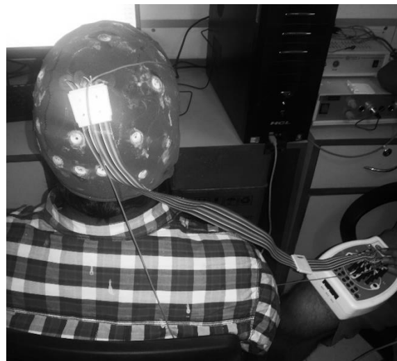
Figure 2. The 32-channel EEG setup used for some experiments of this study
