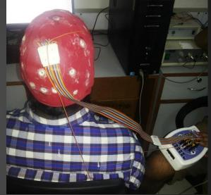
The 32-channel EEG setup used for some experiments of this study
