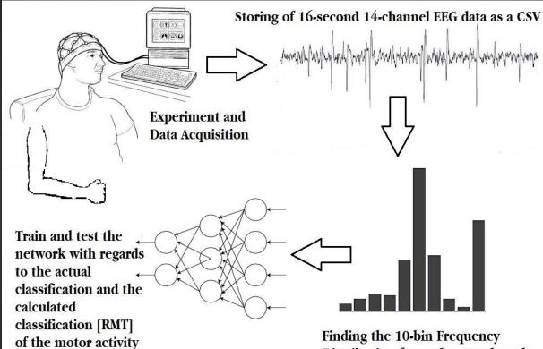
Finding the 10-bin Frequency Distribution for each second, each channel, and forming the appropriate 1X140 vector to be fed into the ANN
